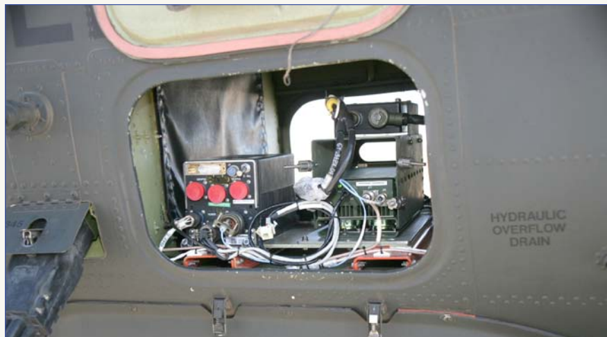
Figure 2 | The AMF JTRS system was placed inside an AH-64 Block III Apache helicopter to test range and capability while relaying voice, data, and imagery from the Apache to ground forces over the Soldier Radio Waveform during an Army Network Integration Evaluation.
